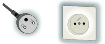
Two round prongs with hole to accept grounding pin.
